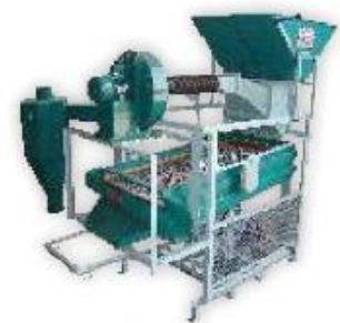
4 x 2 Flat Grader With Cleaner blower system
