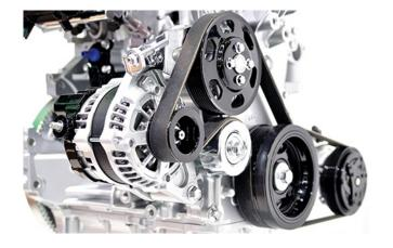
**Automotive Parts (Pulleys)**
